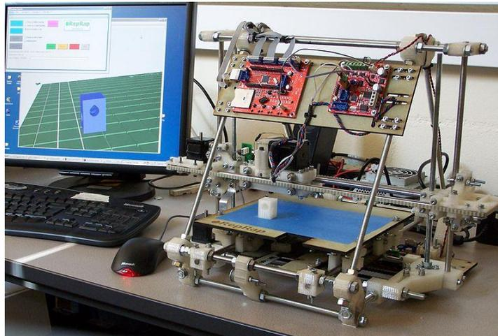
Figure 1: An early RepRap machine (Mendel). Note that all beige components were printed on another 3D Printer with PLA.<sup>1</sup>
