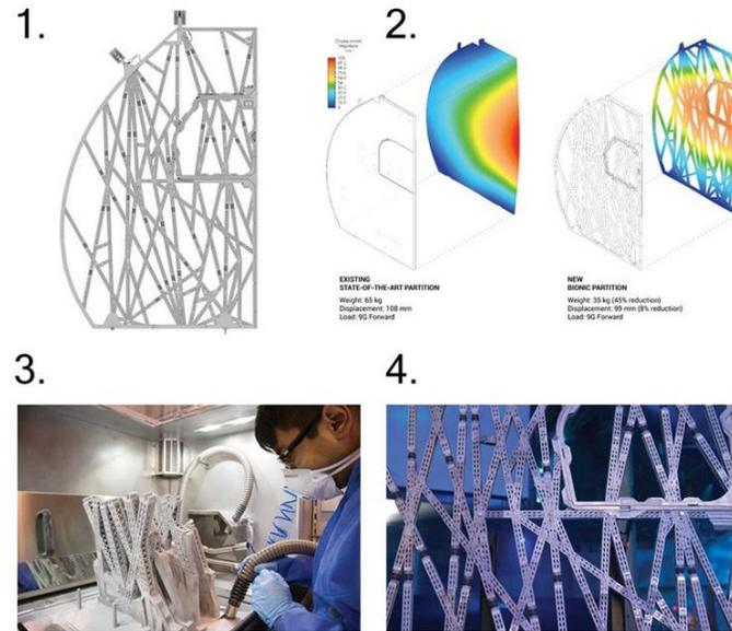
Figure 10: A study of topology optimization to create airplane dividers by Airbus and Autodesk. The final component was 45% lighter and had 8% less displacement.
