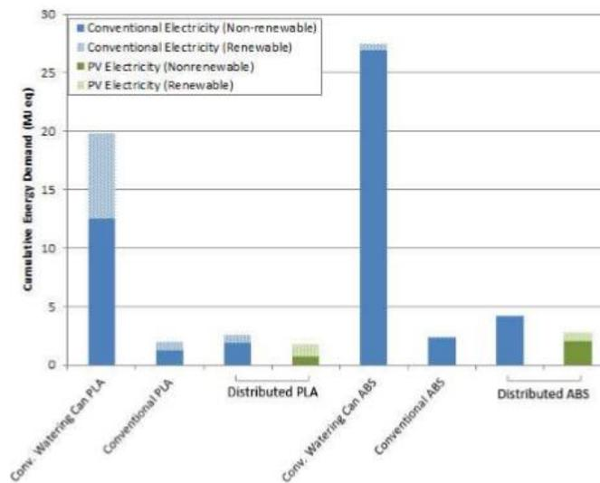
Figure 8: Comparison of overall electricity demand of a high complexity part (waterspout) in PLA and ABS for 3D printing and injection molding. Pearce, et. al.
