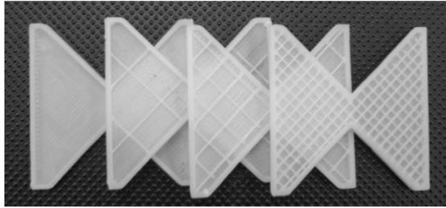
Figure 7: Comparison of infill hatching. From left, 100% 5%, 10%, and 20%. Pearce, et. al.
