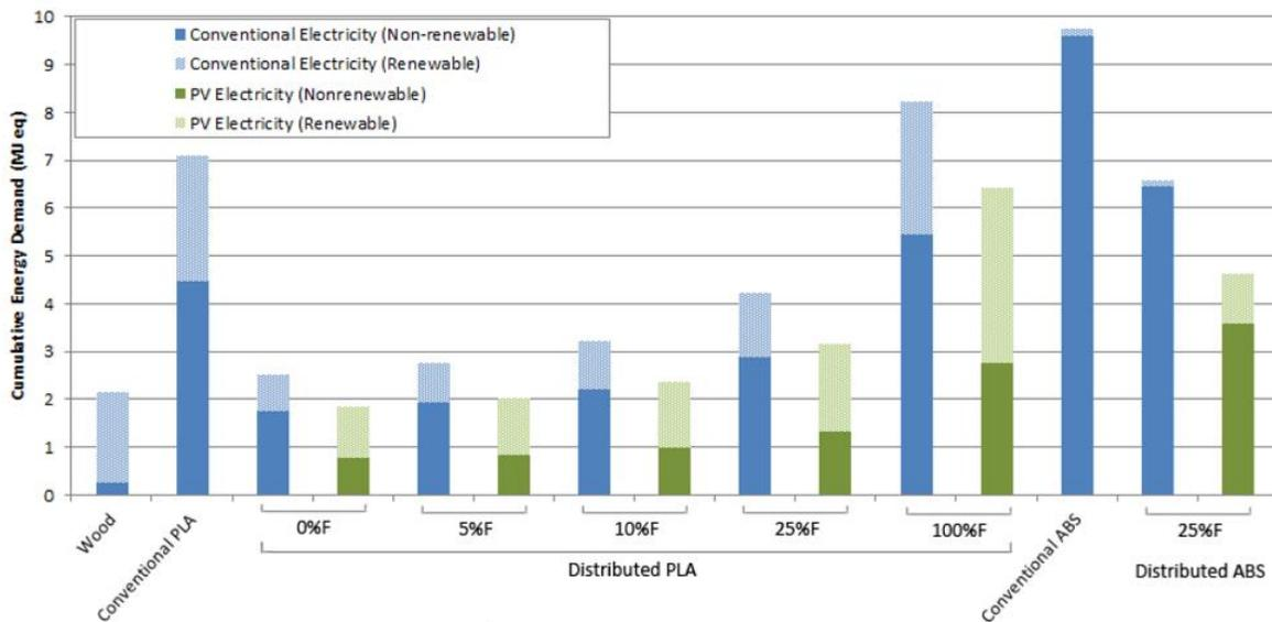
Figure 6: Comparison of overall electricity demand of a low complexity part (block) in PLA and ABS for 3D printing and injection molding. Pearce, et. al.
