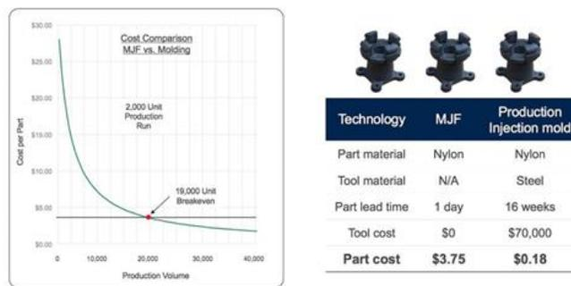
Figure 5: Cost comparison by HP of 3D printing to injection molding. Advancements have made 3D printing cost effective for greater quantities of components.
