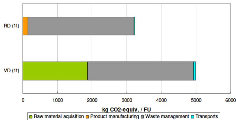
Figure 9: Greenhouse gas emissions estimated by Hiltunen, et. al. from Recycled material (RD) compared to new (VD) for plastic drain covers.
