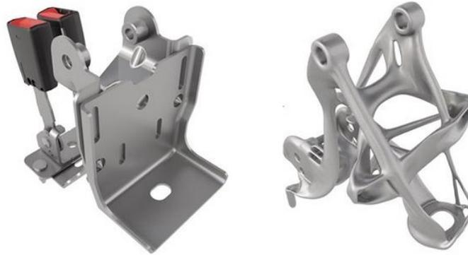
Figure 11: A study of topology optimization for automotive seat brackets by GM and Autodesk. The final component was approximately 40% lighter and 20% stronger.
